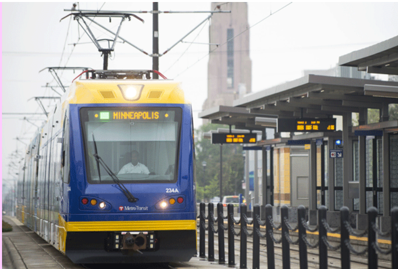
Siemens S70 three-pack heading to Minneapolis - Note sleet pantograph!
